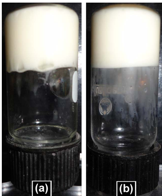
Figure 1. Culture vials containing bigels: (a) G1 (guar gum bigel) and (b) G2 (gum acacia bigel). [Color figure can be viewed in the online issue, which is available at wileyonlinelibrary.com .]
